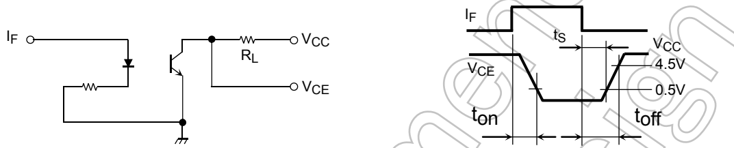
Fig. 1 Switching time test circuit
